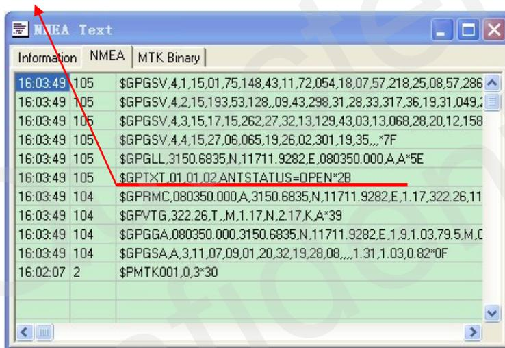
**Figure 17: Patch Antenna Status Description in GPSTXT**
