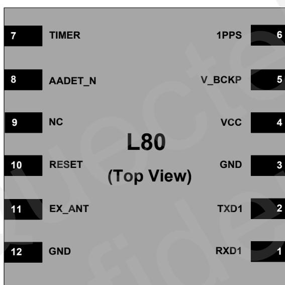
Figure 2: Pin Assignment
