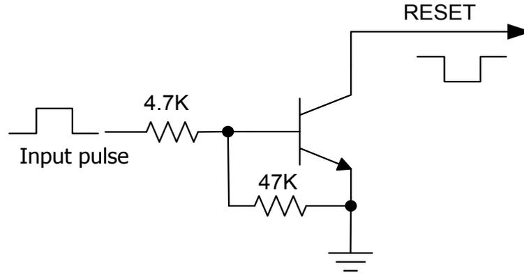
Figure 10: Reference Reset Circuit Using OC Circuit
