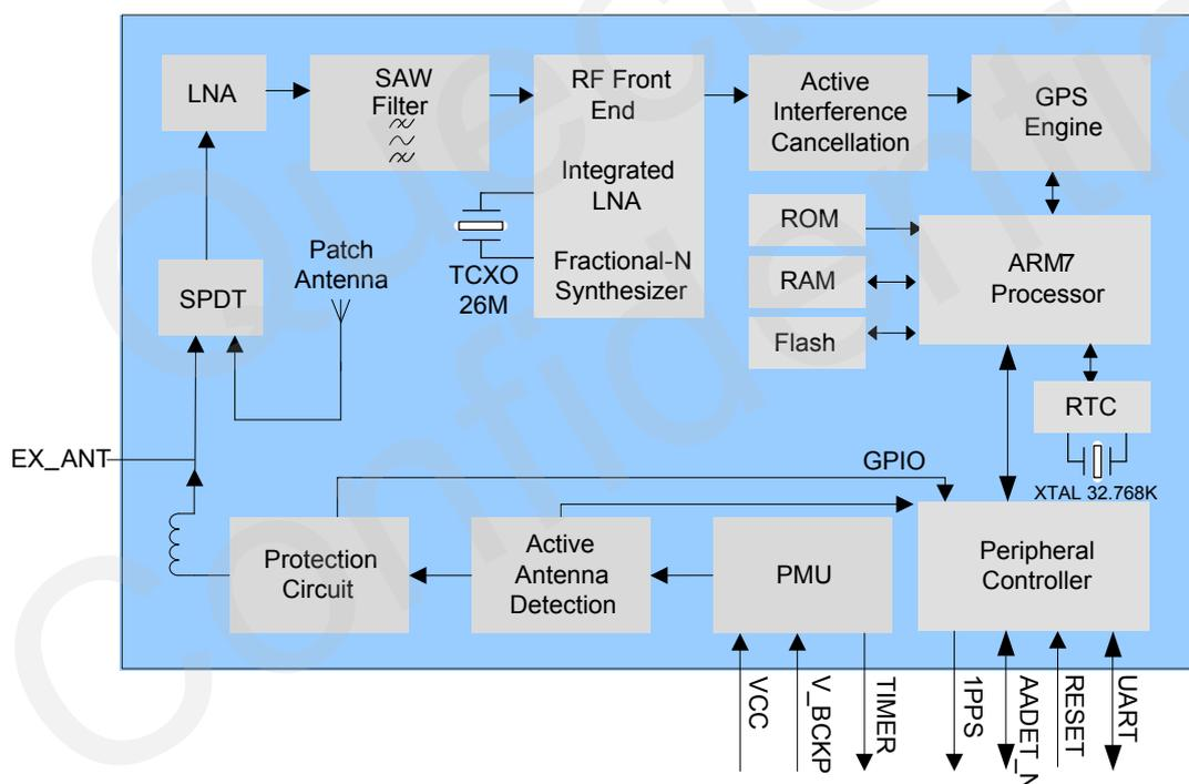
**Figure 1: Block Diagram**
